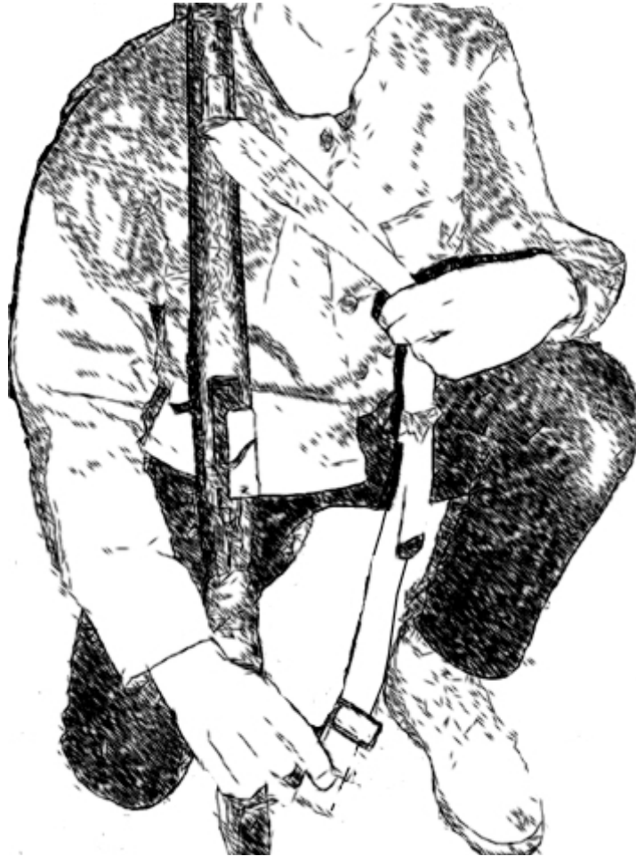
Figure 2. Detach U.S.G.I Web Sling from Lower Sling Swivel.
