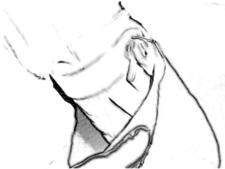
Figure 5. If the hardware is between the mainline and your arm, the sling is on incorrectly.
